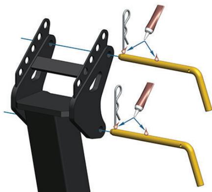
The pivot pins are a vital part of the carrier and with regular applications of a light smear of grease, will slide in and out easily and resist corrosion and wear. The ideal grease is a high quality copper based assembly lube.
