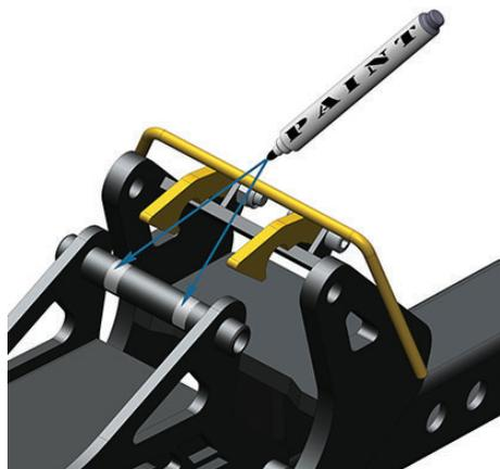
The PoziLock is an over-centre latch that grips the upper pivot sleeve tightly and it is entirely normal for the contact point to be marked. Touch up with a paint pen from time to time. It is not unusual for the latch to pull the upper pin tight when new. The whole pivot assembly has six points of alignment, which requires a bit of travel under load for the pivot assembly to bed in.
