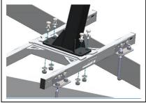
Install the StrongArm support post onto H-Mount flange.
