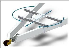
Fine-tune the position of the H-Mount to ensure that the mount is square and set at the ideal position on the drawbar.
