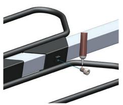
A light application of high quality copper based assembly lube will keep the screws operating easily and allow them to reach the desired tightness by hand. Grease also aids in keeping thread wear to a minimum so apply regularly and wipe off excess.
