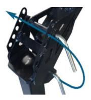
To pivot the carrier assembly up and forwards, remove the lower pin and insert into one of the overhead rotation stop positions. The carrier assembly can then be lifted and pivoted over to the desired stop. This allows easy access to drawbar equipment and to remain attached with bikes loaded.
