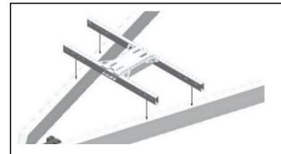
Determine the ideal position of the H-Mount (Item 1) on the drawbar and place the H-Mount (item 1) onto the drawbar.
