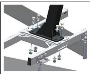
Install the StrongArm support post onto H-Mount flange.
