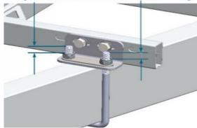
Tighten Nut Pad bolts (Item 7) to 60 Nm torque (really tight).
