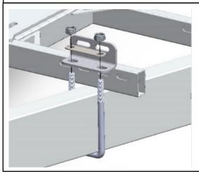
Install U-bolts from underneath the drawbar arms and pass through the shorter slots in the Foot Bracket (item 2). Lower the Washer Shim (Item 4) and retain with the M12 Nyloc Nuts (Item 5).
