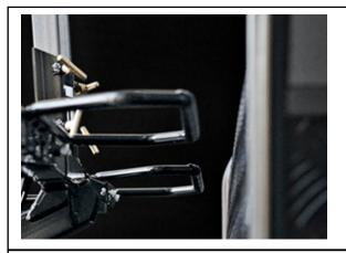
Install the rear wheel support cradles and check clearance to caravan or camper body. Align and adjust H-Mount position and/or slide StrongArm support post fore/aft along slots in cross mount.
